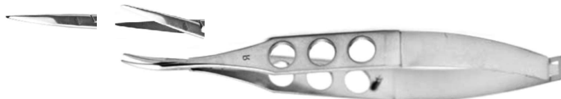
IM-1509 The lower blade of the scissors is thinner and 1mm longer than the upper blade
