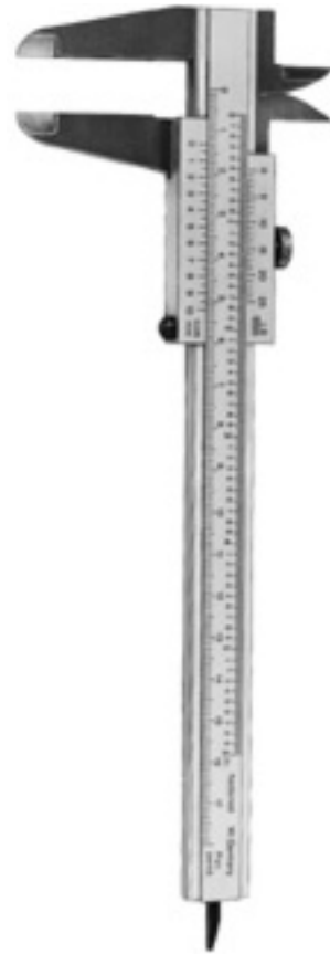
Caliper IM-06-135-21 measuring range up to 200 mm
